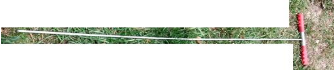
#10. 51.5" axle bar with point on one end and 2" blade on the other-
